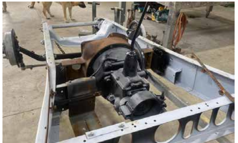
Richard and Terry got all the brakes assembled on the working bee and back on the axles. I machined all the drums back to a fresh new surface for the new shoes, so the brakes on the coffee van should be really nice.
