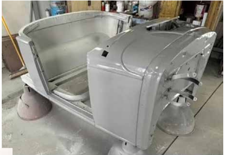
Cowl finished in hi build primer ready for sanding.
