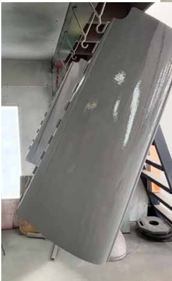
Cowl finished in hi build primer ready for sanding.
