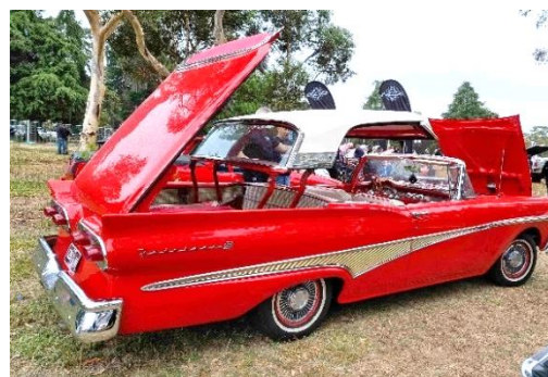
Photo from the All Ford Day, Geelong 2023 showing a retractable roof that is stowed in the 'boot' when not in use
