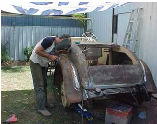
The Chrysler/DeSoto guards being shaped 'in situ' to fit the Plymouth/Chrysler roadster tub.
