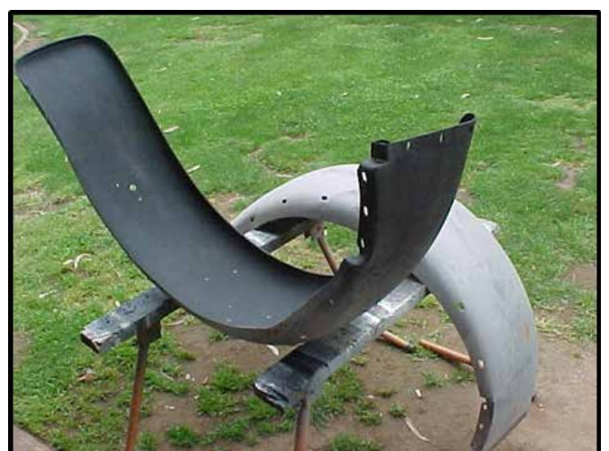
The 'new ' guards, sand-blasted and etch-primed ready for final colour spraying.
